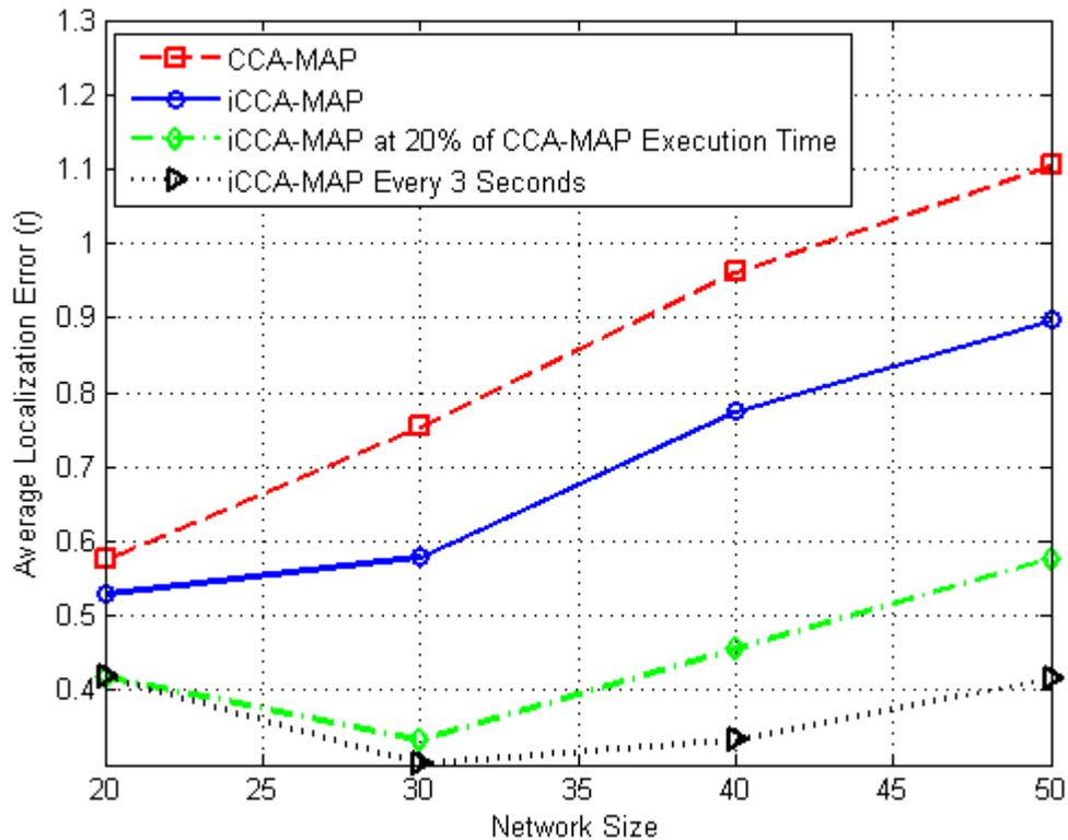
Figure 4-9: Continuous-Time Simulations Comparing iCCA-MAP and CCA-MAP Executed at the Same Frequency and iCCA-MAP Executed at Higher Frequencies.
