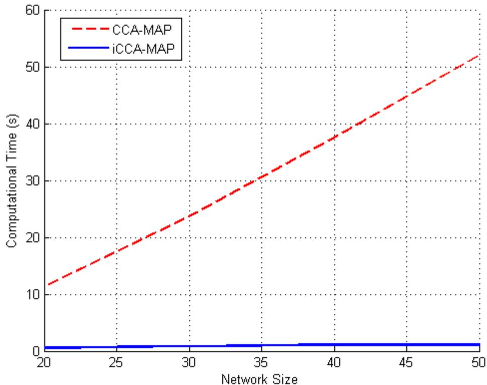
Figure 4-5: Computational Time of iCCA-MAP versus CCA-MAP for Networks of Size 20, 30, 40, and 50 Nodes.
