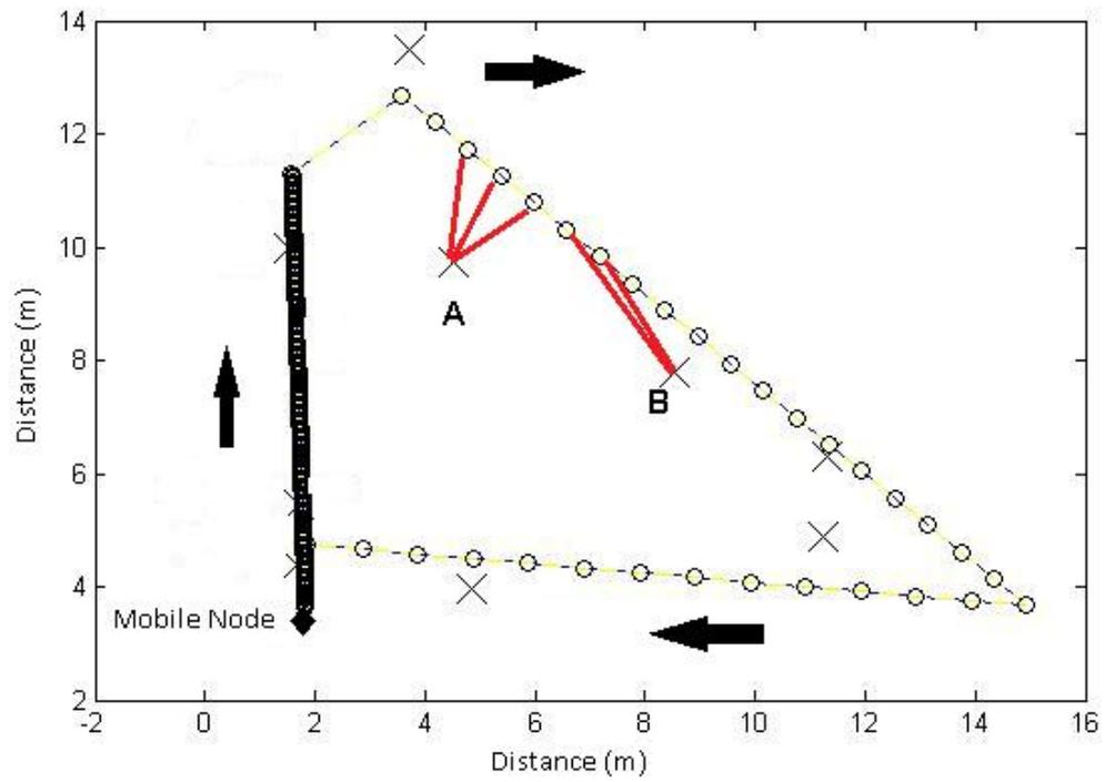
Figure 4-3: Randomly Generated Path Using the Waypoint Mobility Model.
