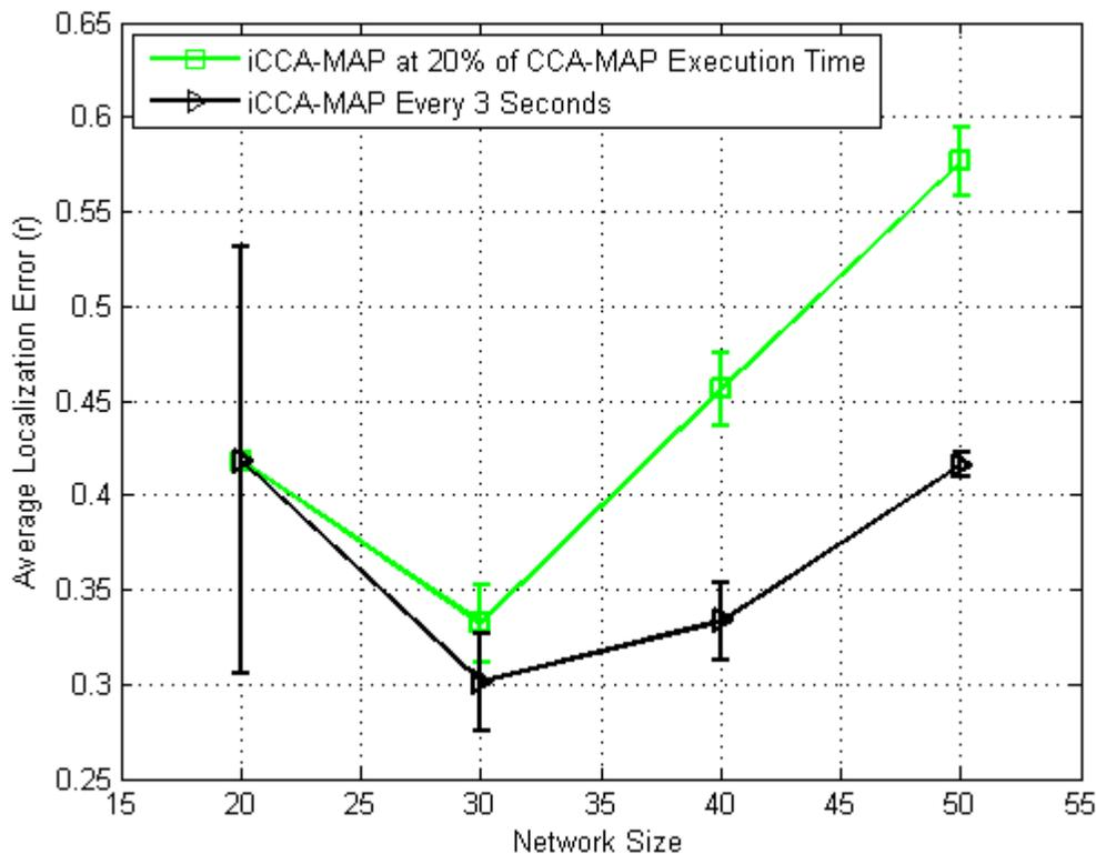
Figure 4-8: Average Localization Error for iCCA-MAP When Executed at 20% of CCA-MAP Execution Time and at Every 3 Seconds in All Cases.
