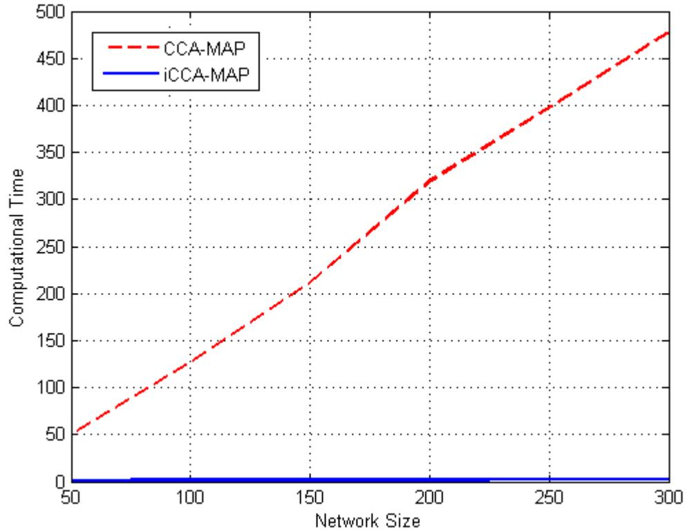
Figure 4-6: Computational Time of iCCA-MAP versus CCA-MAP for Networks of Size 50, 100, 150, 200, 250, and 300.
