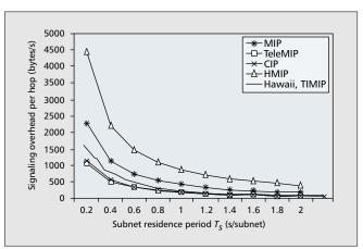
Figure 5. Comparison of total network signaling overhead as obtained in ns-2 (without route optimization).
