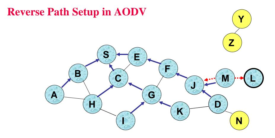
• Node D does not forward RREQ, because node D is the intended target of the RREQ
