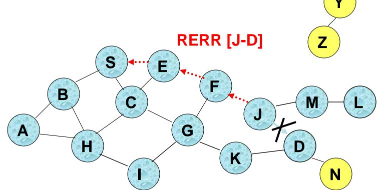
J sends a route error to S along route J-F-E-S when its attempt to forward the data packet S (with route SEFJD) on J-D fails
