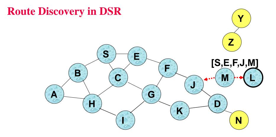
• Node D does not forward RREQ, because node D is the intended target of the route discovery
