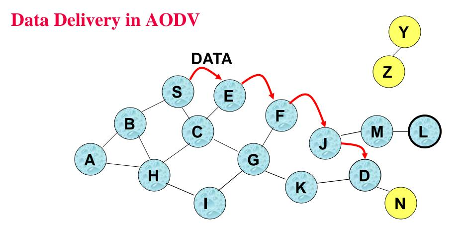
Routing table entries used to forward data packet.
