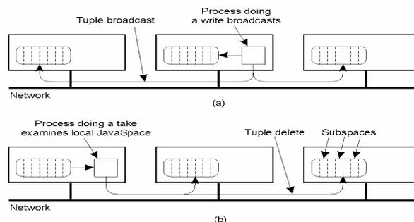
A JavaSpace can be replicated on all machines. The dotted lines show the partitioning of the JavaSpace into subspaces
