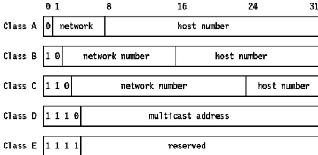
The IP addresses uniquely identify the network and a host on that network
