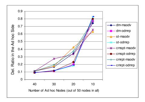
Figure 5.17: Data Packet Delivery Ratio in the Ad hoc Side as a Function of the Subnet Size
