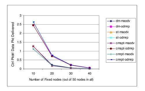
Figure 5.16: Control Overhead per Data Packet Delivered as a Function of the Subnet Size
