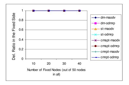
Figure 5.18: Data Delivery Ratio in the Fixed Side as a Function of the Subnet Size
