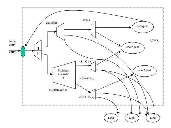
Figure 2.5: Internal Structure of a Multicast Fixed Node in ns-2
