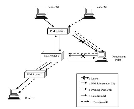
Figure 2.2: Source Specific Tree for Sender S1 and Shared Tree for Sender S2 in PIM-SM
