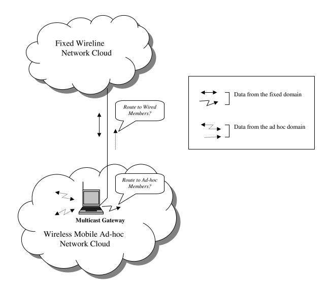
Figure 1.1: Multicasting Between the Fixed and the Wireless Mobile Ad hoc Networks with a Multicast Gateway as an Access Point
